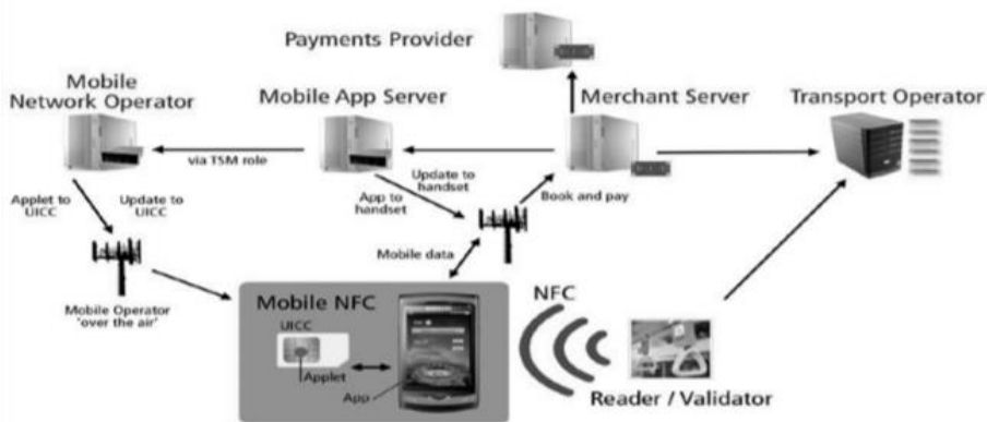
Fig. 4.15. Diagram of interaction between participants in the passenger transport trip accounting system using electronic cards
